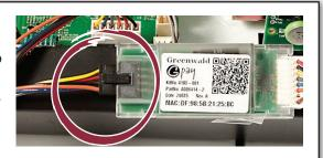
Plug the Greenwald Pay Plus device into the card reader. The Greenwald Pay Pay device is now installed in-between the card reader and the control board.
