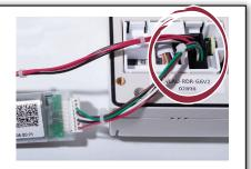
Plug the GPay Plus power cable into the machine control board.
