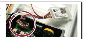
Connect the two power plugs from the Greenwald Pay device to the machines power source (you may need to access these two plugs through the back of the machine.
