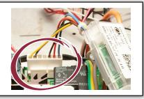
Locate machine power supply transformer and disconnect output power connector.
