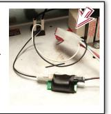
If power supply connector is full, use the IDC splices to attach the power cords.
