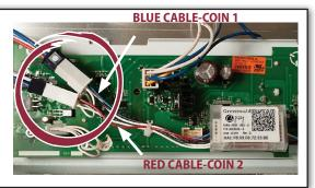
Plug in the serial communication connector on the Greenwald Pay device into the machine control board. "AA3" The Greenwald Pay device is now installed inbetween the coin drop and the control board.
