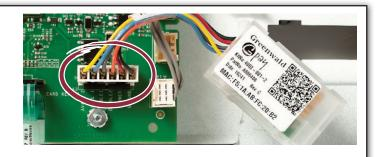
Leave console panel open and re-power the machine. After initialization, the Greenwald Pay device will slow blink white indicating device not configured and is ready to be paired with the profiles set up in GMS.
