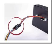
Plug the two pin power connector into the two pin connector on the transformer.
