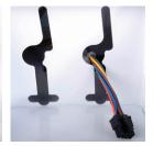
Connect the 8-pin connector to the 8-pin connector of the MultiPav reader.
