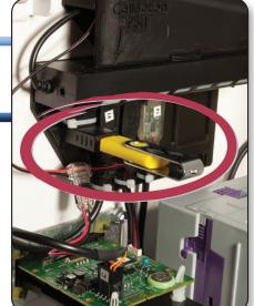
Insert the USB flash drive to disable the vandal features and re-set the cash amount contained in the box to \$0.
