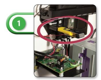
To collect cash and transfer transaction information to GMS, Insert the USB flash drive and select "GET EVENTS AND TRANSACTIONS" from the touch screen > The screen will display "GETTING DATA, DONE" when process is complete
