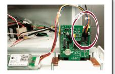
Ensure dip switch #3 is turned on. Leave all other switches in their original positions (change switch position only with power off).
