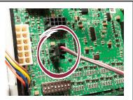
Ensure dip switch #3 is turned on. Leave all other switches in their original positions (change switch position only with power off).
