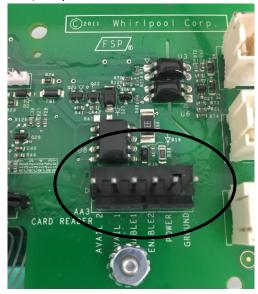
4. (4003-002) (Machines with a coin drop system) The coin system will have to be disconnect from the machine control board and plugged into the Greenwald Pay coin harness. The location of the coin connector on the machine control board will vary, but it will be labeled "COIN1"
