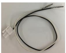
5. Remove coin drop harness or remove coin drop jumper.
