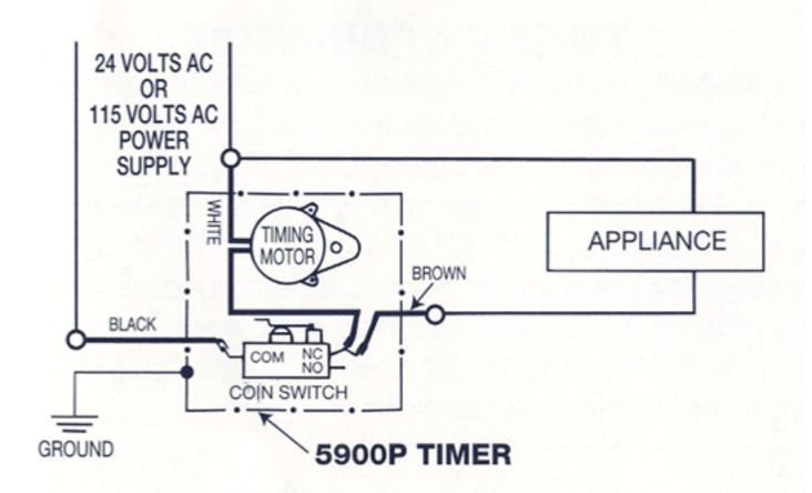
When a coin is deposited, the coin switch closes, activating the timing motor and the appliance. At the end of the total time purchased, the timing motor causes the switch to open, ending the cycle.
