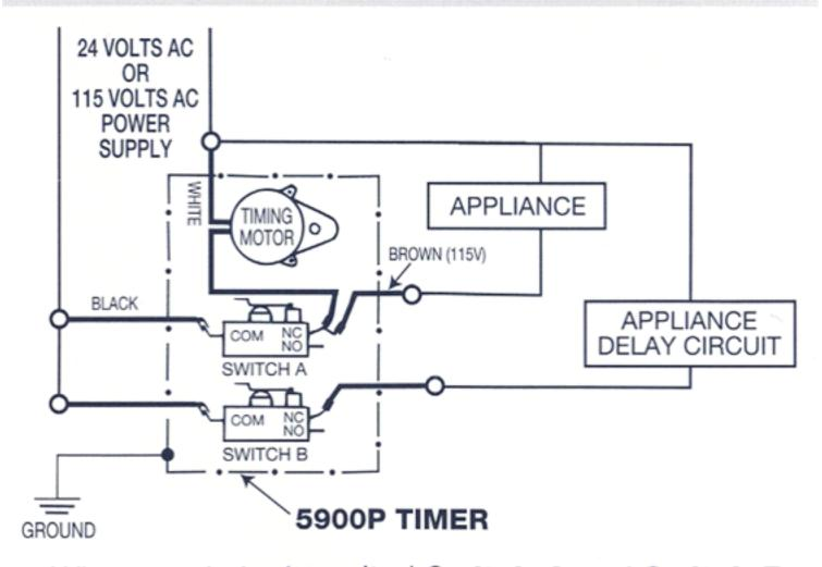
When a coin is deposited **Switch A** and **Switch B** both close, activating both circuits. Toward the end of the cycle **Switch B** opens, shutting off the delay circuit. The main circuit continues to run until the Timing Motor opens **Switch A** ending the cycle.
