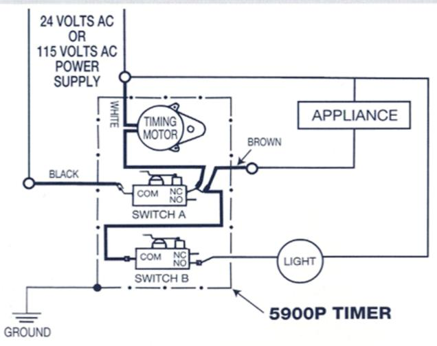
When a coin is deposited **Switch A** and **Switch B** both close activating the appliance. Toward the end of the cycle, **Switch B** transfers to **NO**, activating the light. The appliance continues to run, and the light remains **ON** until the Timing Motor opens **Switch A**, ending the cycle.
